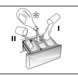
If liquid detergents are used, please insert the special container supplied into the compartment marked "II" in the detergent drawer. This ensures that the liquid detergent enters the drum at the right stage of the wash cycle.
